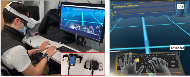
Figure 1: (left) Apparatus consisting of the Quest2 VR headset with a Tobii eye tracker inside, and Tasbi squeeze+vibration wristbands on both hands. (right) Virtual keyboard in VR
